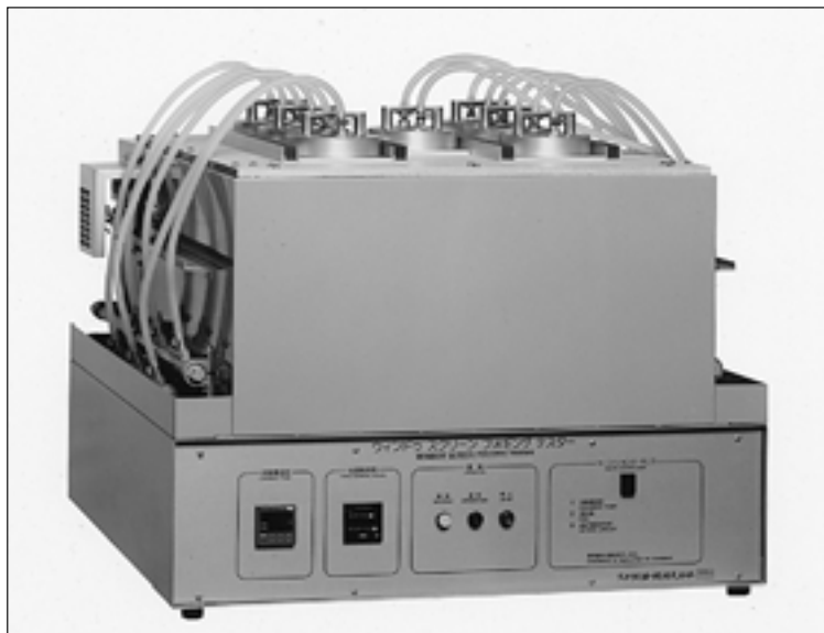
Window Screen Fogging Tester
